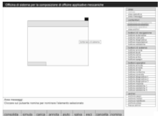
Figure 3. Unwitting programming: the shop foreman drags and drops the entity “bottoniera di sistema” (system button panel) into the canvas representing the background of the line operator environment being created.
