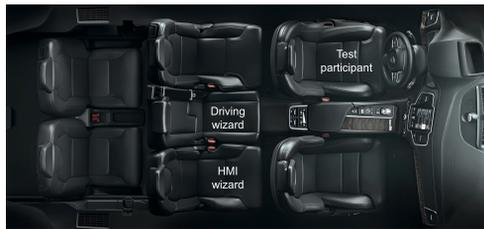
**Fig. 2.** The set-up of the WOz car, which is built on a Volvo XC90. In the set-up, the test participant is positioned in the front seat, and the driving and HMI (Human-Machine Interaction) wizards are positioned in the back seat using driving associated gears and built in displays to simulate autonomy. A test leader can be positioned in the front or in the back, depending of its role in the study.
