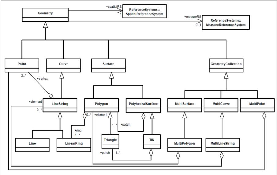
Fig. 3. OGC Geometry class hierarchy.
