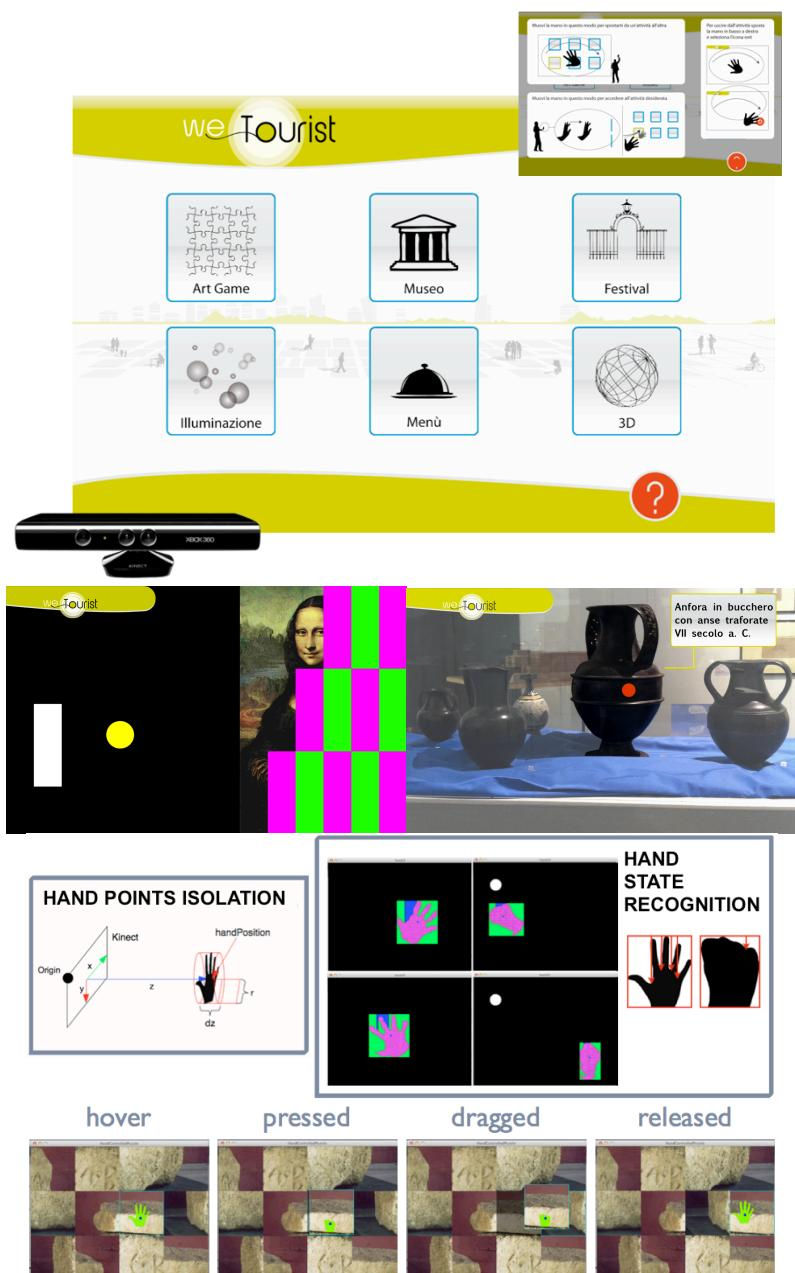
**Fig. 6.** Prototype of PoInt, Kinect based, containing games and informative widgets. The two interaction strategies adopted are also illustrated.
