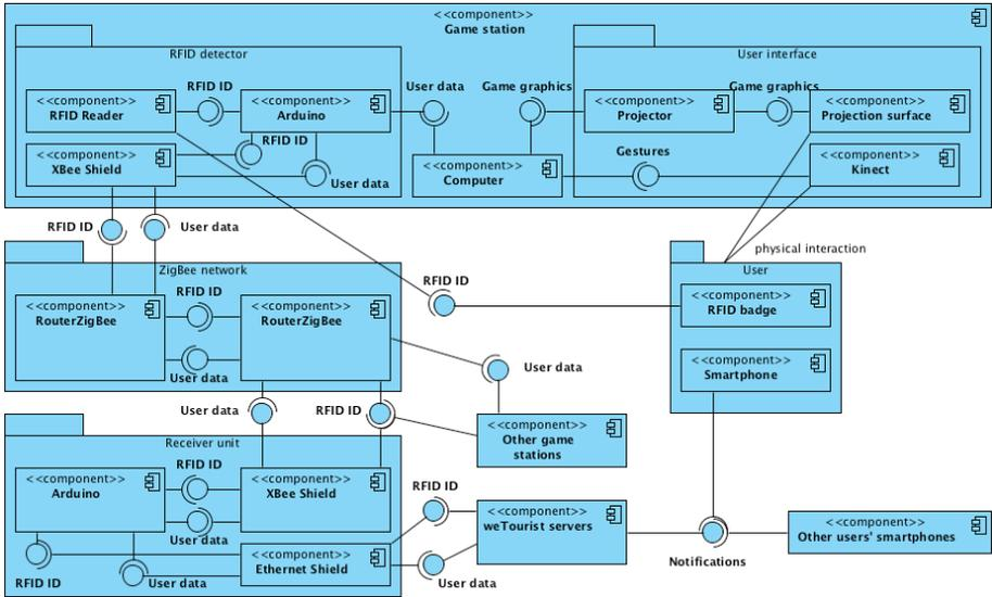
**Fig. 5.** UML diagram of a typical PoInt
