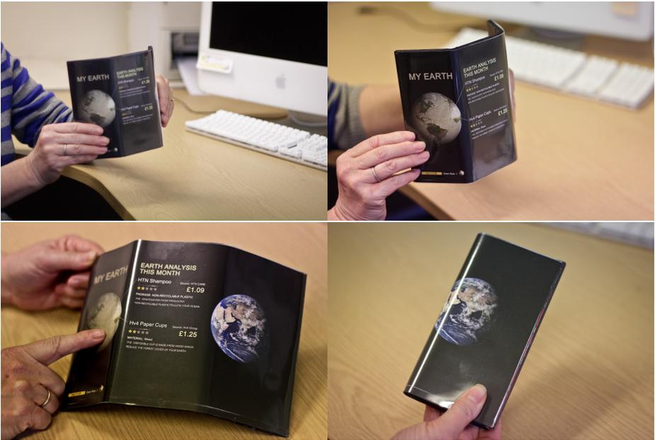
**Fig. 4.** Four views of a (prototype) folding tablet computer
